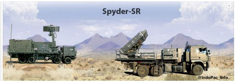
SPYDER SR has 360° engagement capability. Missiles can launch in less than 5 seconds from target confirmation. The kill range is from under 1km to 20 km and at altitudes from 20 m to 9 Km. The SPYDER SR command & control unit has a built in EL/M-2106 ATAR radar. SPYDER SR carries 4 missiles per firing unit. The missile firing units use a slant missile launcher.
