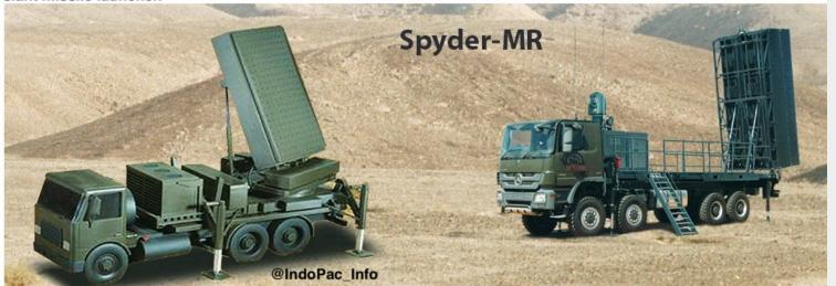
SPYDER MR has 360° engagement capability. Missiles can launch in 2 seconds from target confirmation. The kill range is up to 40 km and to 16 Km altitude. SPYDER MR has a separate radar unit using the larger, more powerfull EL/M-2084 radar. SPYDER MR carries 8 missiles per firing unit. The missile firing units use a vertical missile launcher.
