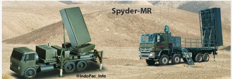
SPYDER MR has 360° engagement capability. Missiles can launch in 2 seconds from target confirmation. The kill range is up to 40 km and to 16 Km altitude. SPYDER MR has a separate radar unit using the larger, more powerfull EL/M-2084 radar. SPYDER MR carries 8 missiles per firing unit. The missile firing units use a vertical missile launcher.
